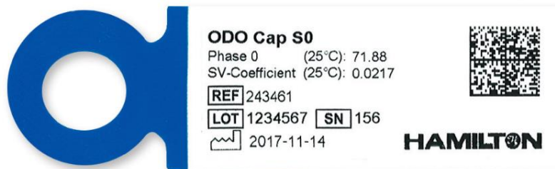
Figure 15: Example sensor label with calibration data
